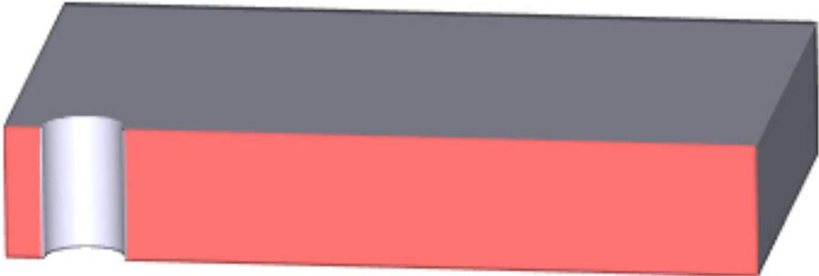
A solid with section turned on, the axis is created as axis of hole.
