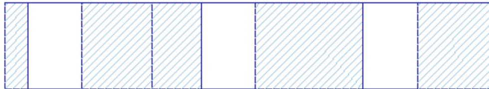
Created hatches of 3D section. After changes of 3D model, these hatches are rebuilt automatically.
